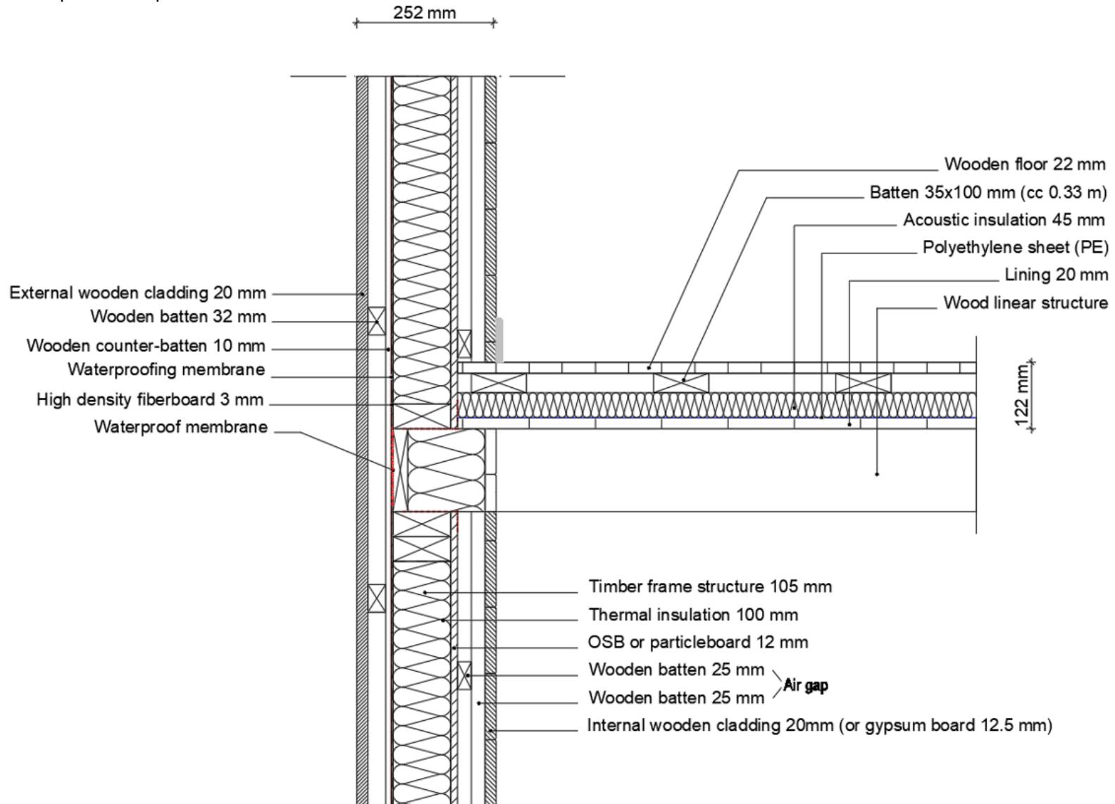
15 – TFS 145 – Floor panels composed of linear wood strucutre
